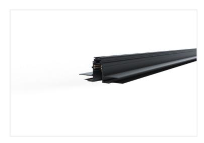
Trimless Mounting DC48V Voltage **Dimensions** (W) 103mm x (H) 54mm 2000mm Length Finish Black Material Aluminium Driver Remote IP Rating IP20 Accessories Out Corner Warranty 5 years
