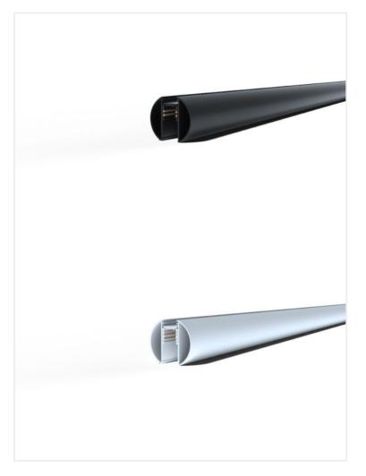
Mounting Surface, Suspended Voltage DC48V **Dimensions** (W) 59mm x (H) 54mm Length 2000mm **Finish** Black, White Material <u>Aluminium</u> Driver **Remote IP Rating** <u>IP20</u> Accessories **Control Gear** Warranty 5 years <u>Track Mounted – Tracks & Accessories</u> **Luminaires Type**
