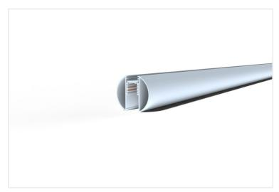
Mounting Suspended DC48V Voltage (W) 59mm x (H) 54mm Dimensions 2000mm Length Finish White Material Aluminium Driver Remote IP Rating IP20 Accessories
