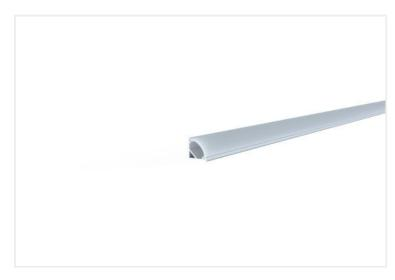
Micro Mounting (W) 10mm (H) 10mm Dimensions 2000mm Length Finish White **Extrusion Material** Aluminium Diffuser Material Polycarbonate **End Cap Material** Polycarbonate Warranty 5 years **Luminaires Type** Linear Systems - Profiles
