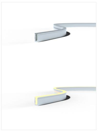
Wattage 10W/m Voltage DC24V **Dimensions** (W) 6mm x (H) 12mm **Cut Length** <u>25mm</u> CCT 2700K, 3000K, 3500K, 4000K Beam Angle <u>160°</u> Driver **Remote IP Rating** <u>IP67</u> **Luminaires Type** <u>Linear Systems - Linear Light Source</u> **Luminous Flux** 150lm CRI <u>>92+, >98</u> **Colour Deviation** <3 SDCM Accessories **Control Gear** Warranty 5 years 1-500lm Luminous Flux lm
