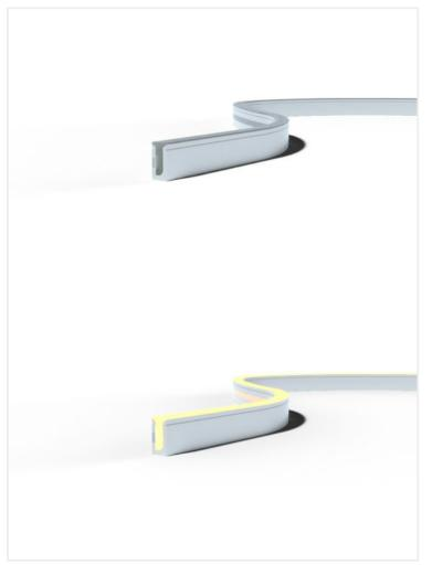
Voltage DC24V **Dimensions** (W) 6mm x (H) 12mm **Cut Length** <u>25mm</u> CCT 2700K, 3000K, 3500K, 4000K **Beam Angle** <u>160°</u> Driver **Remote IP Rating** <u>IP67</u> **Luminaires Type** <u>Linear Systems - Linear Light Source</u> **Luminous Flux** 150lm CRI <u>>92+, >98</u> **Colour Deviation** <3 SDCM Accessories **Control Gear** Warranty 5 years 1-500lm Luminous Flux lm
