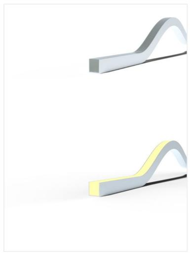
Wattage 15W/m Voltage DC24V **Dimensions** (W) 16mm x (H) 17mm **Cut Length** <u>55.5mm</u> 2700K, 3000K, 3500K, 4000K, 5000K, RGB, Solid Colours CCT Beam Angle Driver **Remote IP Rating** <u>IP67</u> **Luminous Flux** <u>950lm</u> CRI <u>>83+</u> **Colour Deviation** <3 SDCM Accessories **Control Gear** Warranty **Luminaires Type** <u>Linear Systems – Linear Light Source</u> Luminous Flux lm 501-1000lm
