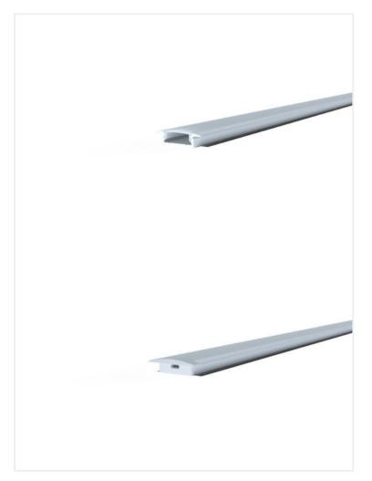
Mounting Recessed **Dimensions** (W) 18.5mm x (H) 7mm Length 2000mm, 2500mm, 3000mm Anodized Aluminium, Black, Custom Powdercoat, White **Finish Extrusion Material** <u>Aluminium</u> Diffuser Material **Polycarbonate End Cap Material Polycarbonate** End Caps, PC Diffuser, PC Diffuser (Black) Accessories Warranty <u>Linear Systems - Profiles</u>
