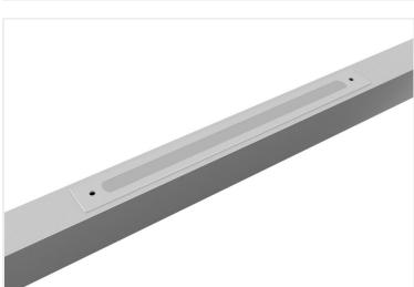
Mounting Wattage 1.5W Voltage DC24V Dimensions (W) 17.5mm x (H) 21mm x (L) 185mm 30 x 30mm square handrail with 0.8-3mm wall thickness **Suitable Locations Finish** Stainless Steel CCT 3000K Beam Angle Symmetric Material Stainless Steel **IP Rating** IP67 **Luminous Flux** 140lm CRI >83+ **Colour Deviation** <3 SDCM Lifetime 50,000 hours Warranty 5 years
