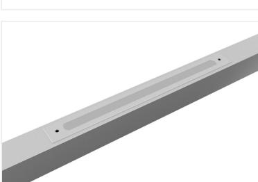
Mounting Wattage 1.5W Voltage DC24V Dimensions (W) 17.5mm x (H) 21mm x (L) 185mm 30 x 30mm square handrail with 0.8-3mm wall thickness **Suitable Locations Finish** Stainless Steel CCT 4000K Beam Angle Symmetric Material Stainless Steel **IP Rating** IP67 **Luminous Flux** 140lm CRI >83+ **Colour Deviation** <3 SDCM Lifetime 50,000 hours Warranty 5 years
